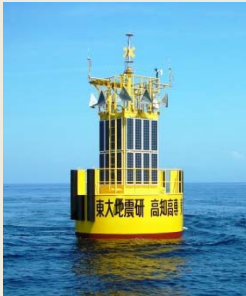
GPS Tsunami Monitoring System
