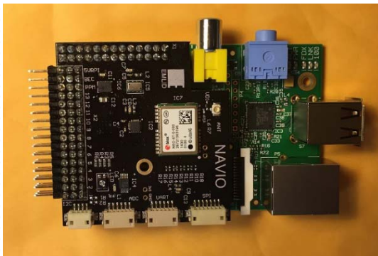
NAVIO: Autopilot Shield for Raspberry Pi ($195 + $40) http://www.emlid.com/
