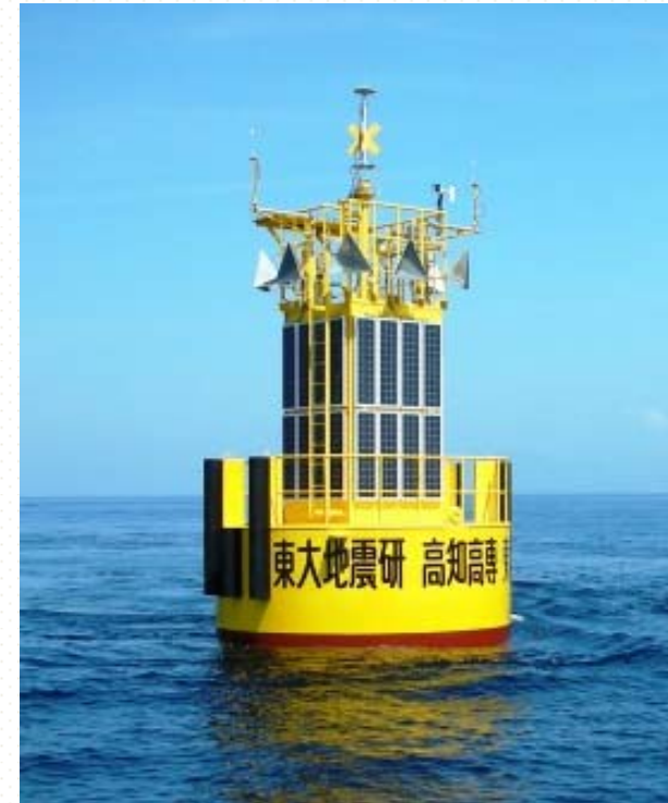
GPS Tsunami Monitoring System (Currently ~15 km off-shore)
