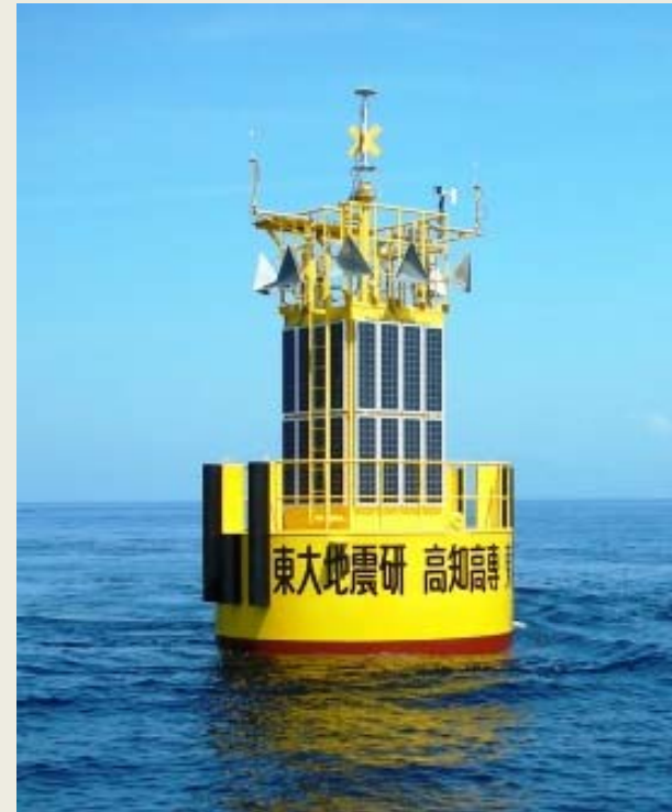
GPS Tsunami Monitoring System (Currently ~20 km off-shore)
