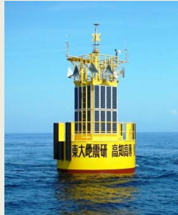
GPS Tsunami Monitoring System (Currently ~15 km off-shore)
